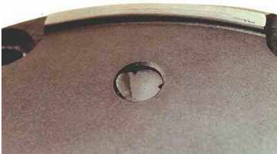
II-3-3-5. Dowel pin cut in two
